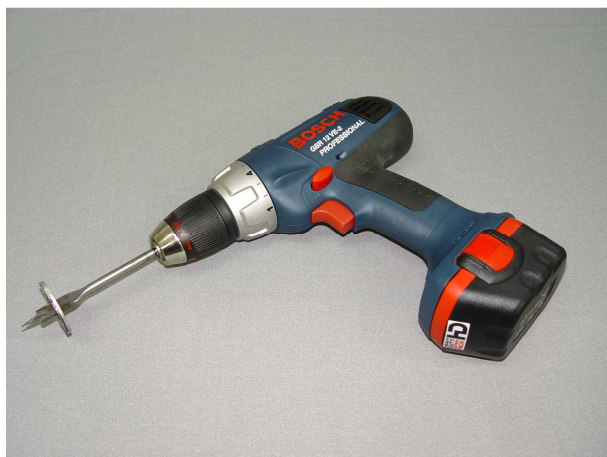
Photo No 9 Cordless drill with a bit to make filling holes 25 mm in diameter
