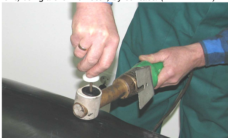
Photo No 57 Heating up to achieve softening of the filling hole edge and the plug conical surface by means of a plug welder
