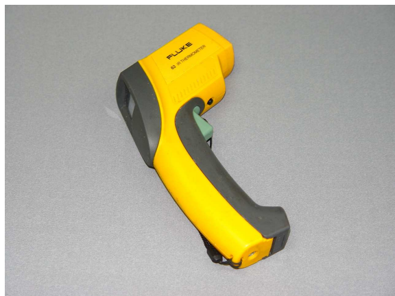
Photo No 7 Pyrometer to measure temperature of heat-shrinkable sleeve - recommended
