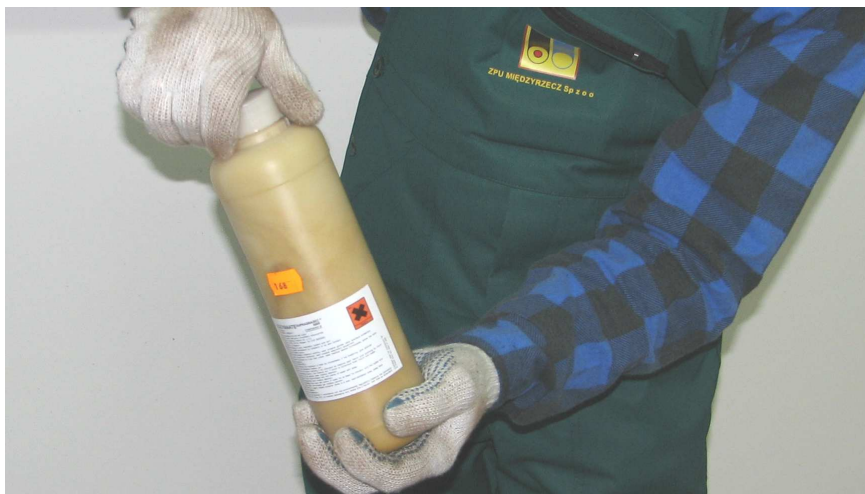
Photo No 48 Mixing of Components A and B of the PUR foam
