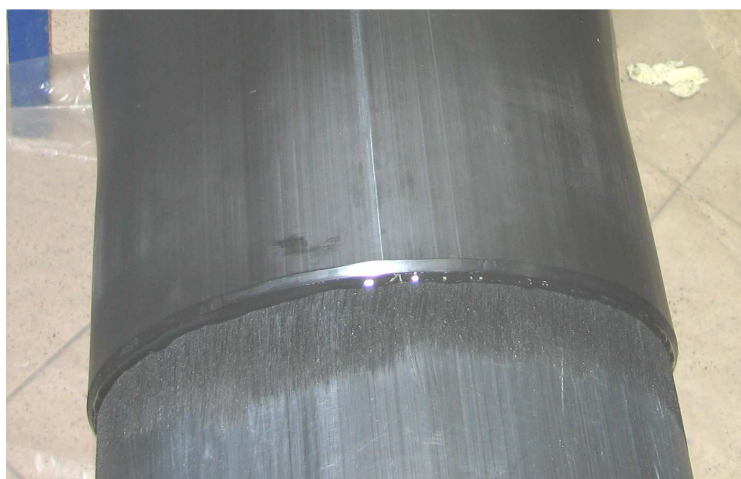
Photo No 32 View of adhesive binder flashes at the edge of the heat-shrinkable sleeve – the circumference of the pre-insulated pipe
