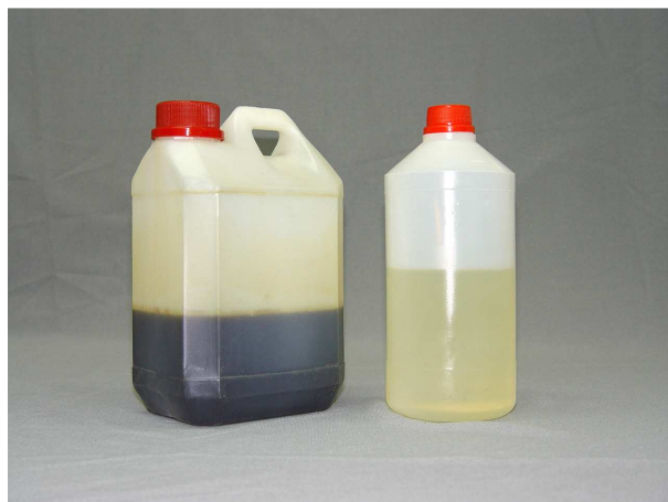
Photo No 19 PUR foam (Component A+B)
