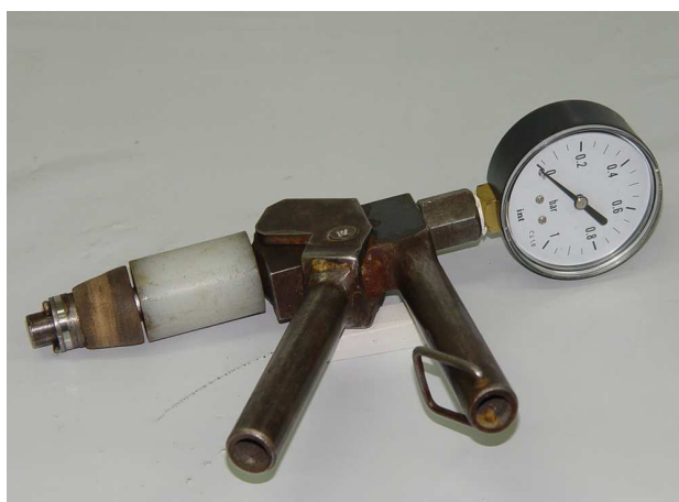
Photo No. 11 Test manometer with expansion cap
