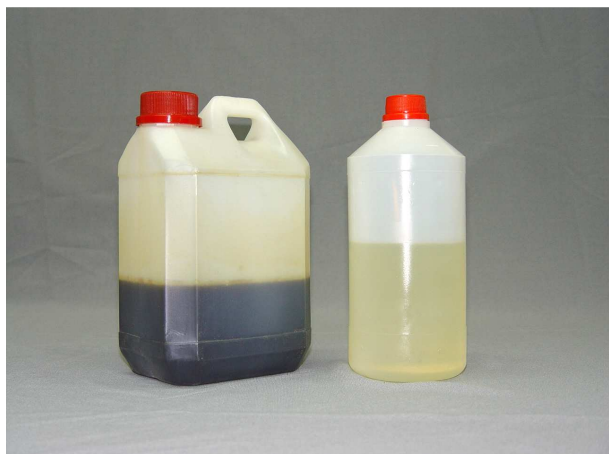
Photo No. 18 PUR foam(component A+B)
