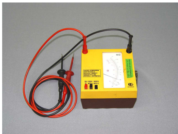
Photo No. 15 Resistance measurement gauge
