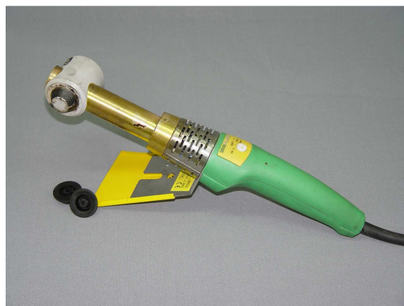
Photo No 8. Welding machine for plugs
